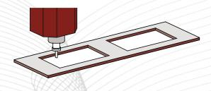
POLISHING OF THE TOP AND OF THE EDGE WITH POLISHING PADS
