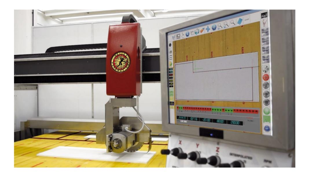
The Photoscan system is the digital camera over the Helios machines. With the integrated Run-touch 1.0 software, the precision Photoscan system digitizes and measures the slab just with one picture. It manages the cutting processes with the macros, improves the arrangement and management of a slab warehouse (scraps and remnants included), and works also as a template reader. Moreover, it has the Vein-Matching App for the complex layouts that need to follow the natural flow of the material.
